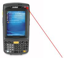
Hold Down the red On/Off button in the top right hand corner for 5 to 10 seconds until the screen shows MC70 Warm Boot. Once it reboots try Logging into Scannabar.
