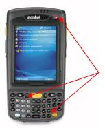
ii. Do this by holding down the red On/Off button in the top right, and the number 1 & 9 on the keyboard. All buttons must be pressed down at the same time.
