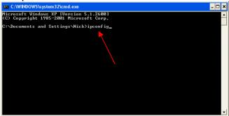
5. This will now display the IP address currently assigned to your PC. Write this down. In this example we have an IP of 172.17.1.101
