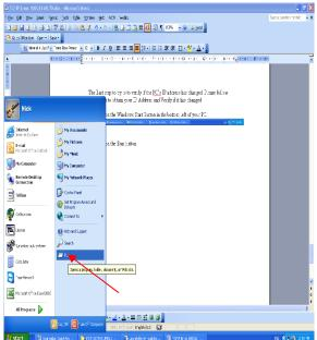
3. The Run box should open up. In the Open field type CMD or COMMAND and click OK
