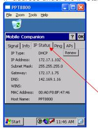
What we are looking for here is weather we have a Static or DHCP address. Once we see that we should see an address populate the IP address field. If you see 0.0.0.0 then you are not properly setup on your network and will need to contact your Network administrator to setup your Handheld Scanner.
