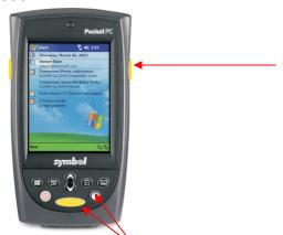
1. Press on the Enter and Half Moon icon as well as the Yellow trigger on the top right hand side. All buttons must be pressed down at the same time. If you have done this correctly you will see a Symbol PPT8800 Screen.
