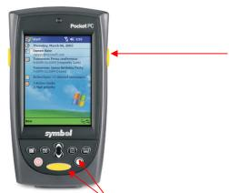
Press on the Enter and Half Moon icon as well as the Yellow trigger on the top right hand side. All buttons must be pressed down at the same time. If you have done this correctly you will see a Symbol PPT8800 screen.
