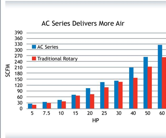
AC Series offers you the next level of sophistication. Featuring industry leading CFM performance, quiet {as low as 67 dB(A)} operation, electronic controllers, energy saving soft-start Wye-Delta motor starters, TEFC motors, air-cooled aftercoolers and optional integrated refrigerated air dryers.
