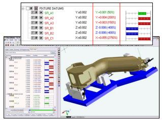
The fixture adjustments calculated by CheckMate to balance the stock on the casting to optimize the machining process are used to adjust the fixture prior to machining
