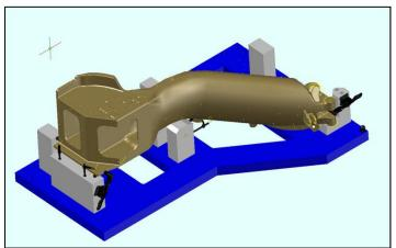
In this CheckMate screen shot the corrective action required to adjust the fixture prior to machining is calculated using SoftFIT Solver and clearly presented in the Root Cause Browser.
