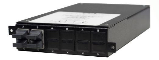
Network test access points (TAPs) are hardware tools that allow you to monitor your network. All fiber breakout TAPs are passive, purpose-built hardware devices that make a 100% copy of your network's data allowing your monitoring tools to see every bit, byte and packet.®
