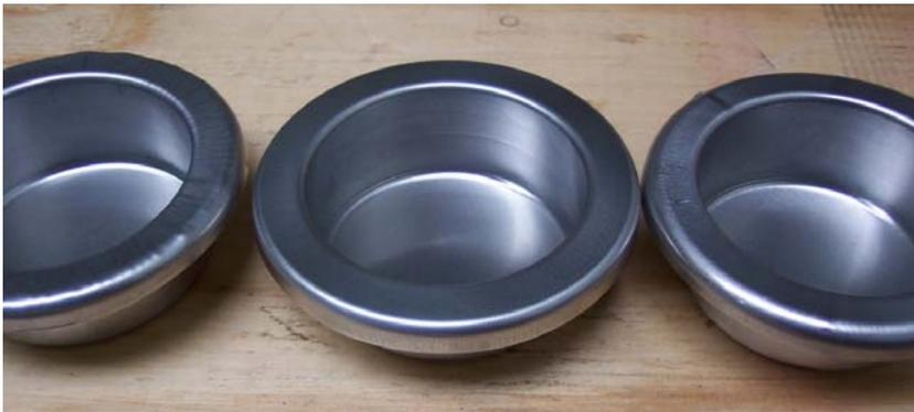
**Figure 15. Wrinkling in half-formed cup (left, right) and satisfactory cup (middle).**
