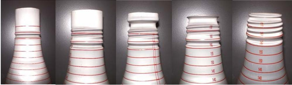
**Figure 9. Top-finish forming operations: tamper-band forming, threading, pre-curling, trimming, and curling**
