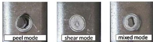
**Figure 2: Fracture modes for resistance spot welds**
