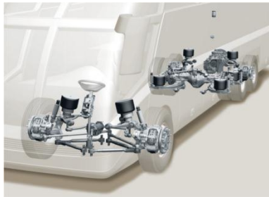
Figure 1. Suspension for a tri-axle passenger bus. (ZF, 2012)
