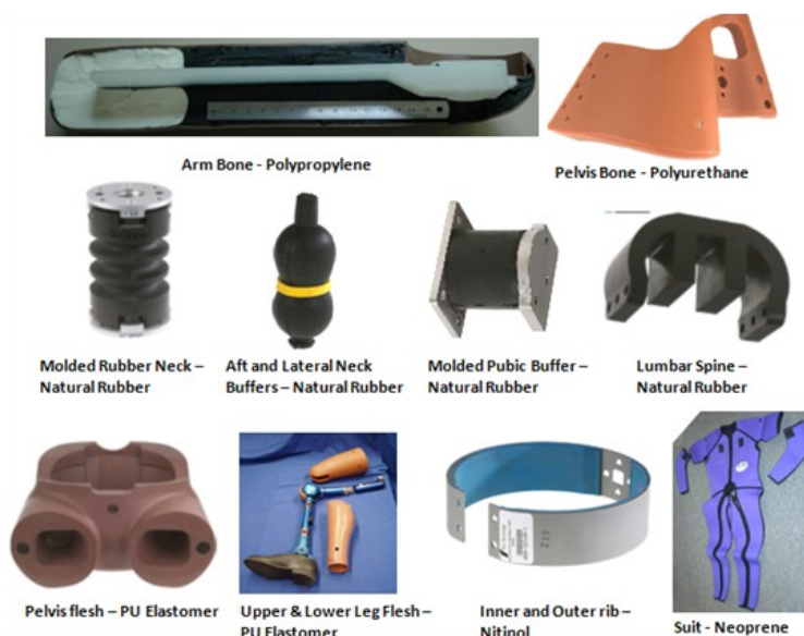
Figure 1: Components and materials of the WorldSID 50 dummy
