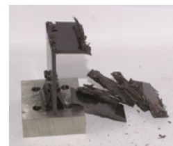
Figure 4. Example of CFRP material exhibiting poor crushing behavior.
