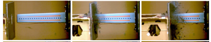
Figure 2. Dynamic impact loading on a CFRP cone structure.
