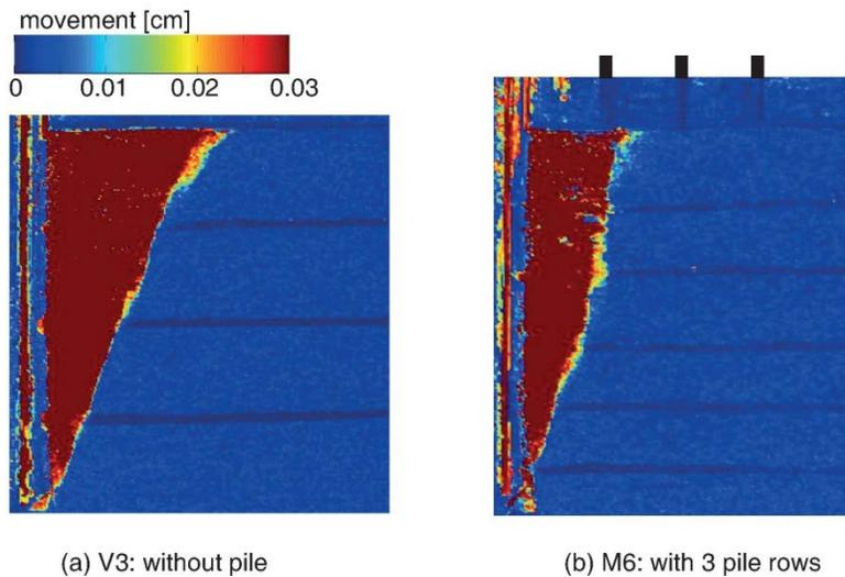
**Figure 6. Contour plots of the soil movement at critical state with PIV approach: (a) Test V3 without pile; (b) Test M6 with 3 pile rows [17]**
