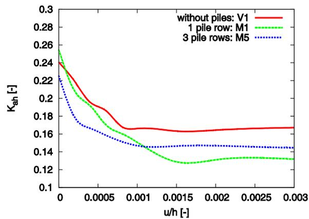
**Figure 4. Relationship between  $K_{ah}$  and the relative wall movement  $u/H$  due to parallel translation of the wall**
