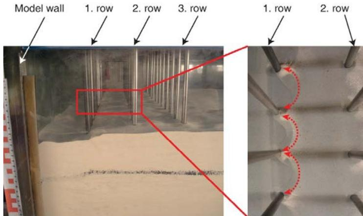
**Figure 5. Side (left) and top view (right) of test M6 after a parallel translation of  $u/H = 0.012$  [17]**
