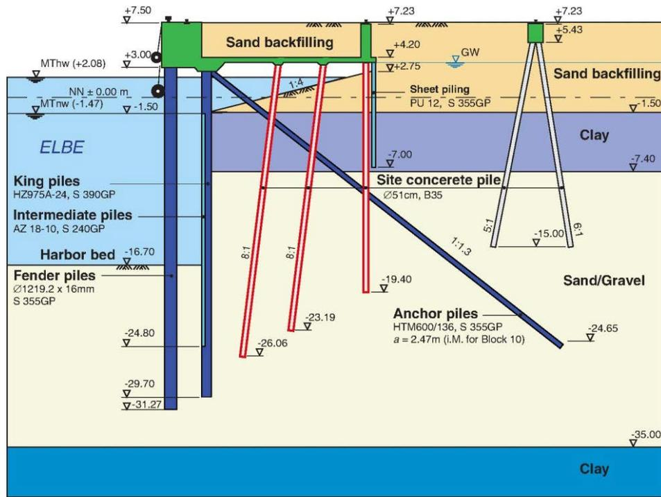
**Figure 1. Section of the quay structure Containerterminal Alterwerder (CTA) in Hamburg, Germany [1]**
