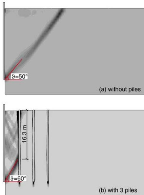
**Figure 8. Development of shear band due to parallel movement of the wall;  $H=25\text{m}$ ,  $L=2\text{m}$ ,  $d=0.5\text{m}$ ,  $b=b_1=5\text{m}$ ; (a) without piles, (b) with 3 piles [28]**
