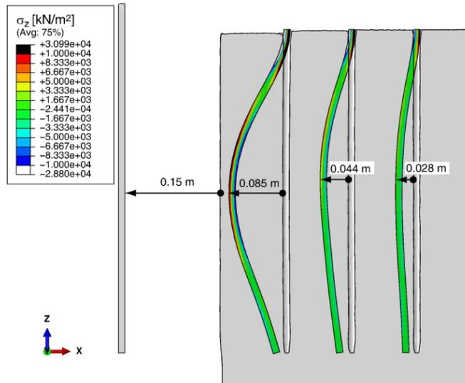
Figure 9. Deformed piles (deformations scale factor =50) due to parallel movement of the wall;  $H=25\text{m}$ ,  $L=2\text{m}$ ,  $d=0.5\text{m}$ ,  $b=b_1=5\text{m}$ ,  $u/H=0.006$ , with 3 elastic pile rows
