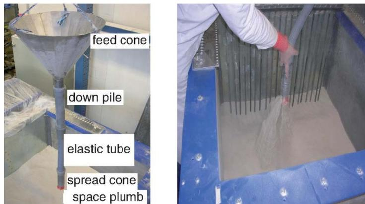
**Figure 3. (a) Feeding device; (b) Filling of the bin [16]**
