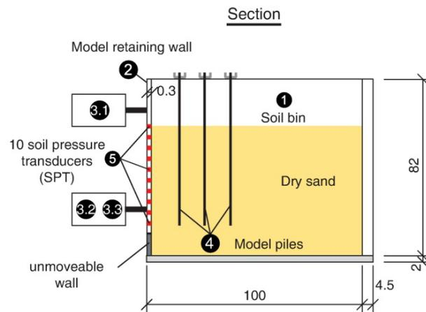
**Figure 2. Test stand of the 1g model test to investigate the earth pressure on the model retaining wall, unit [cm]**
