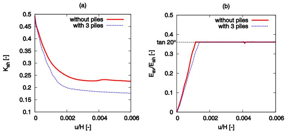
Figure 10. Deformed piles (Relationship between (a)  $K_{ah}$  and (b)  $E_{av}/E_{ah}$  and the relative wall translation  $u/H$ ;  $H = 25\text{ m}$ ,  $L = 2\text{ m}$ ,  $d = 0.5\text{ m}$ ,  $b = b_1 = 5\text{ m}$ )
