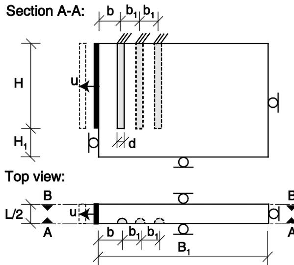
**Figure 7. Geometry and boundary conditions of the FE-simulations used for analyzing the earth pressure on a retaining wall**
