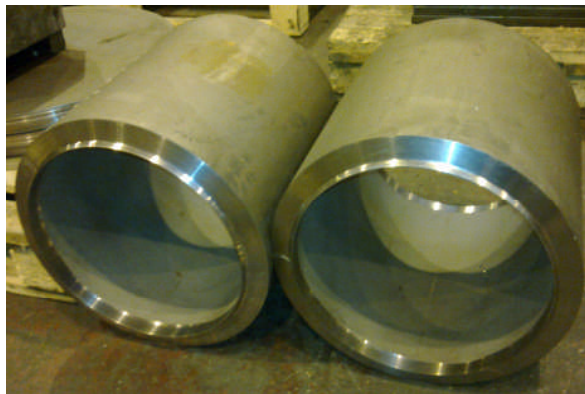
Figure 1. P92 pipe before welding.
