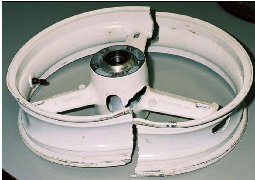
Figure 1. Damaged motorcycle wheel.
