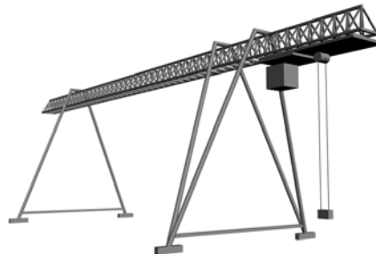
Figure 9. General arrangement of the subject portal crane.
