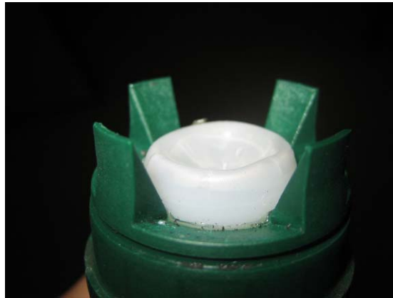
Figure 2. Collapsed lens cover
