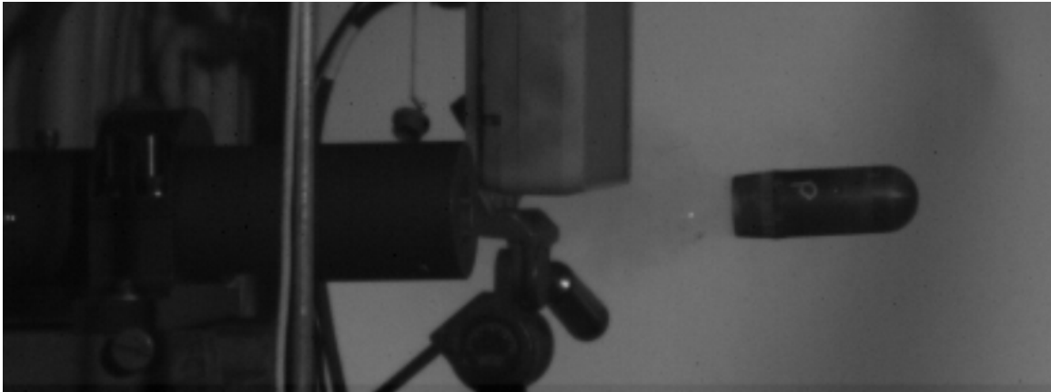
Figure 16. High speed photo at muzzle exit during live fire test
