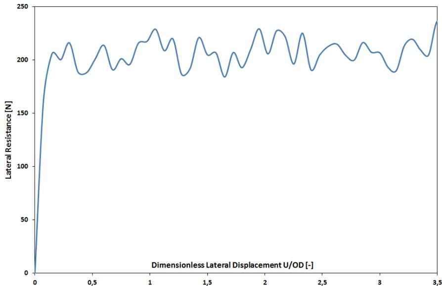
**Figure 5. Lateral resistance during pipeline break-out**
