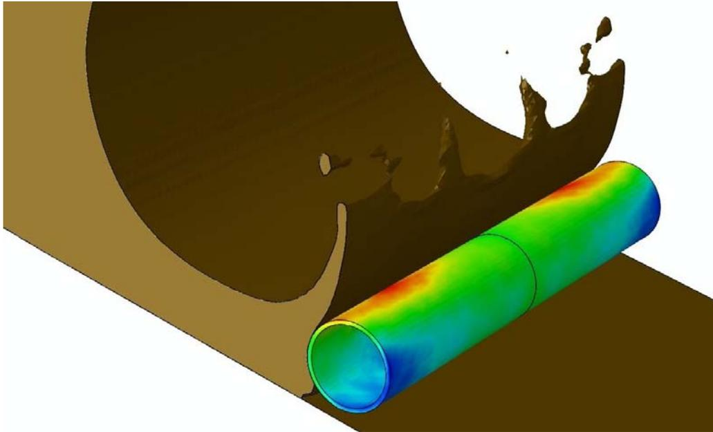
**Figure 11. Impact induced stresses during full-scale submarine debris flow impact**
