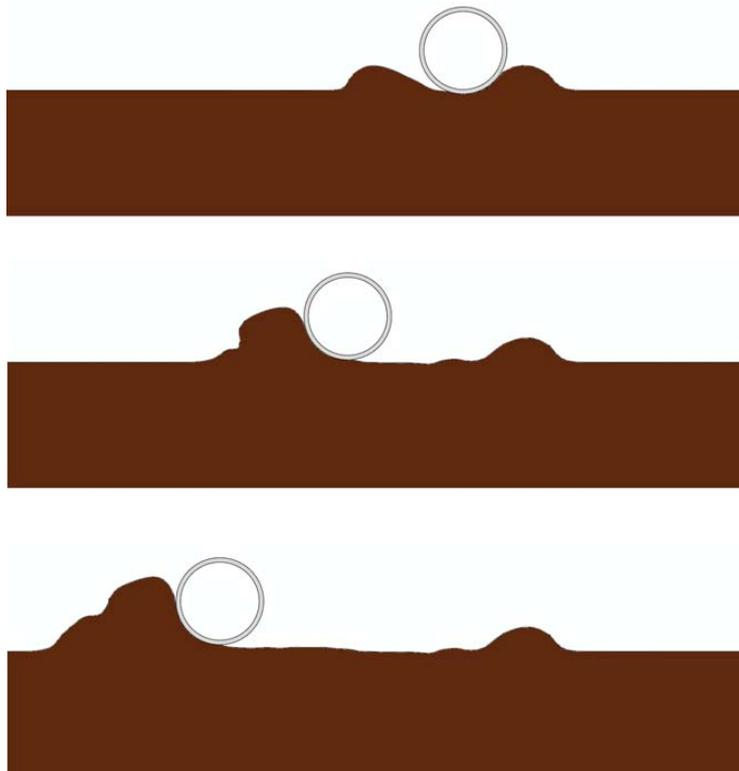
**Figure 4. Cyclic lateral movement, berm formation and break-out**
