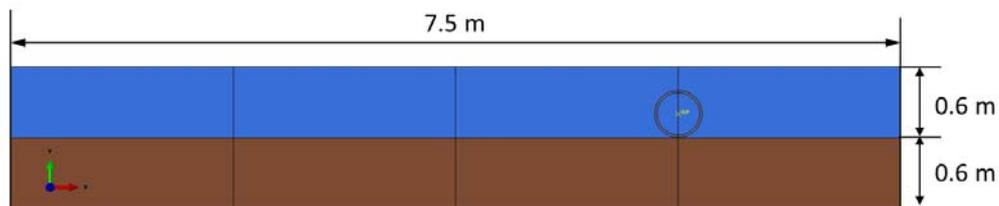
**Figure 1. Definition of the Eulerian domain: rigid subsea pipeline on seabed soil**
