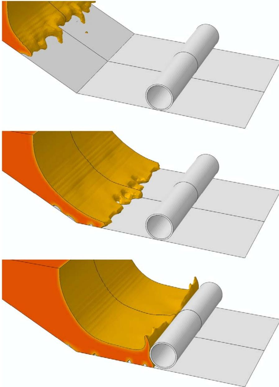
**Figure 10. Submarine debris flow impact on large diameter pipeline**
