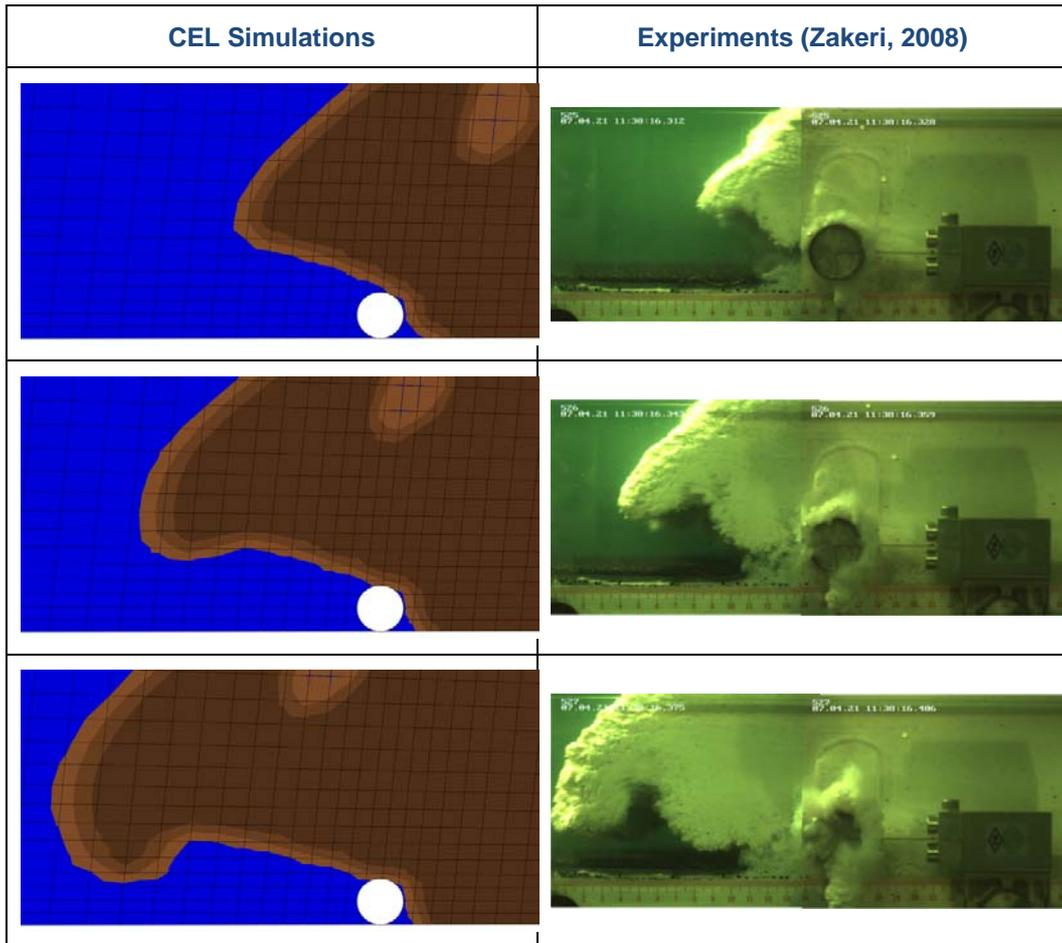
**Figure 8. Submarine debris flow impact: CEL simulations vs. experiments**
