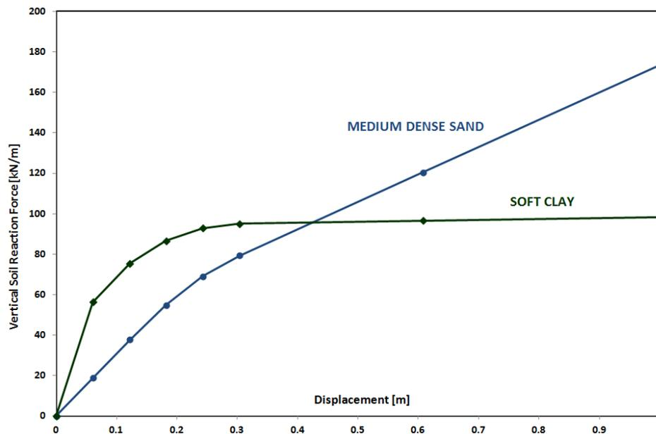
Figure 13. Vertical soil reaction for sand and clay
