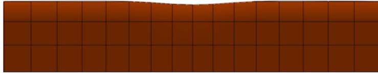
**Figure 3. Initial pipeline embedment under gravity loading**
