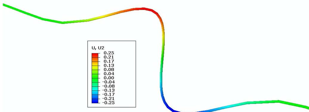
**Figure 14. Lateral buckling of subsea pipeline during operation**
