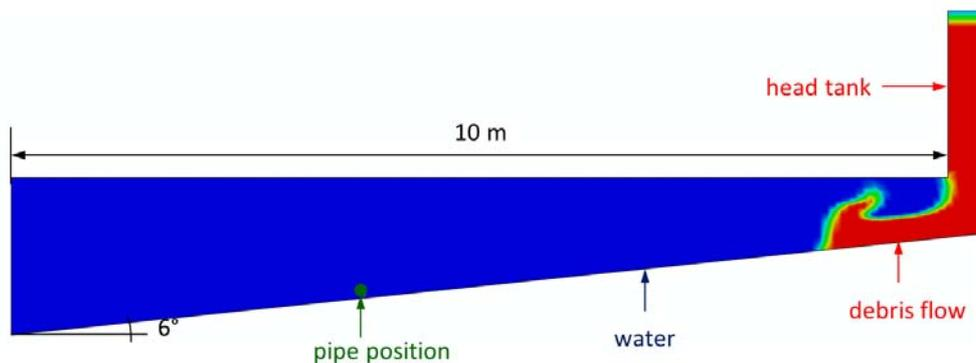
**Figure 6. CEL model to simulate submarine debris flow impact on pipelines**
