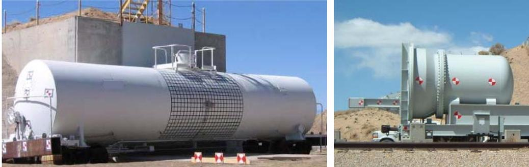
**Figure 3. Tank and ram cars in a shell impact test.**
