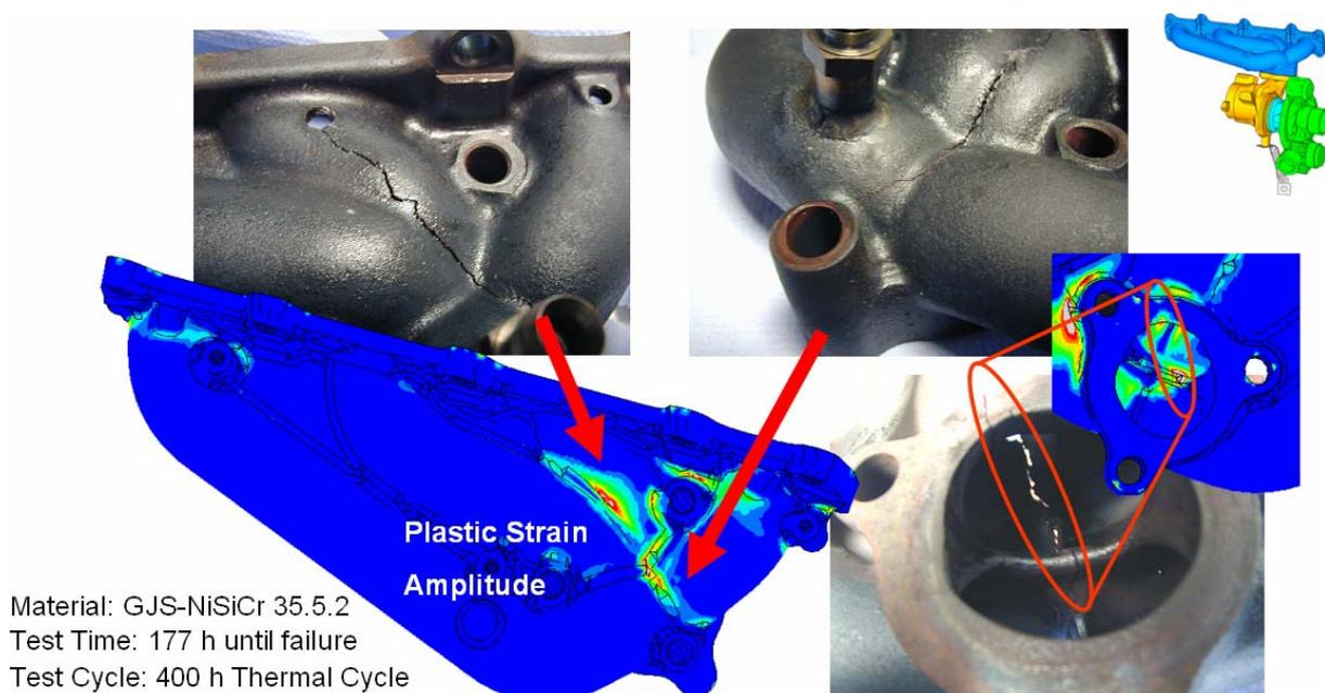
**Fig. 7 Comparison simulation and hardware at an early design stage**
