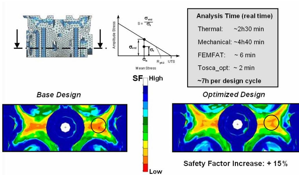
**Fig. 5 Comparison HCF-results of base and optimized structure**
