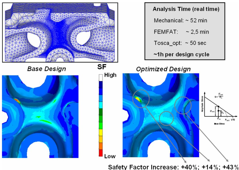
**Fig. 6 Comparison HCF-results base and optimized structure at the sub-model**
