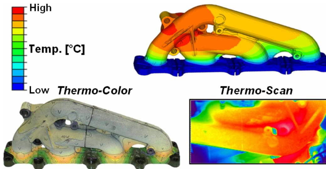
**Fig. 8 Temperature distribution from simulation and measurement**
