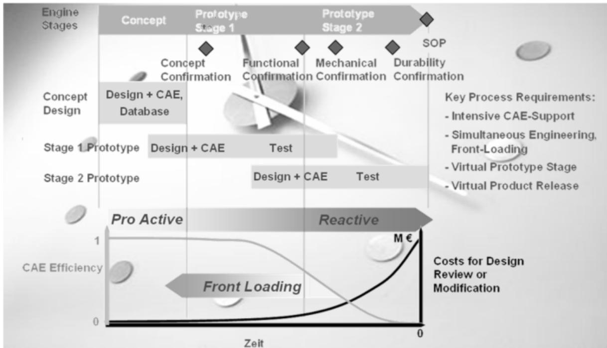
**Fig. 1 Simultaneous CAE in the development plan**
