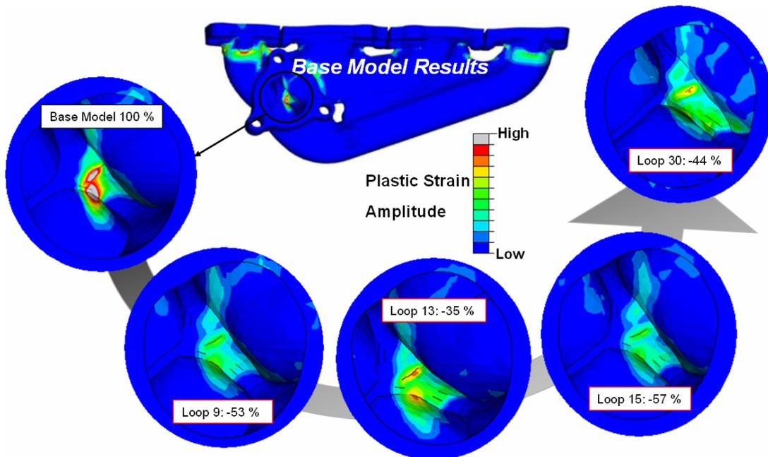
**Fig. 9 Optimization results via cycles**
