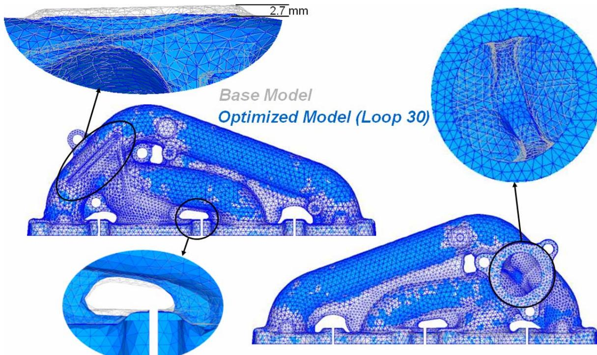
**Fig. 10 Comparison basis and optimized geometry**
