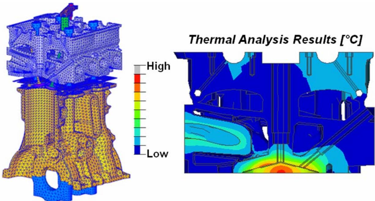
**Fig. 3 FE-model with temperature distribution**
