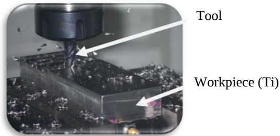
Figure 2. The material and the tool used in the test.
