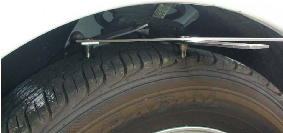
Figure 2 - Experimental setup of spike pull test
