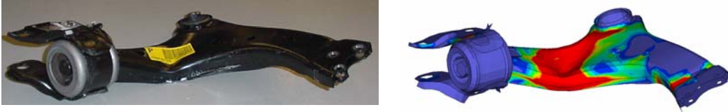
Figure 11a. Impact Rig Buckling - TEST. Figure 11b. Impact Rig Buckling - CAE.
