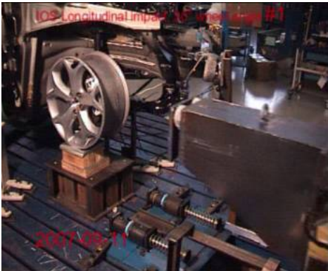
Figure 10a. Susp Impact - TEST.
