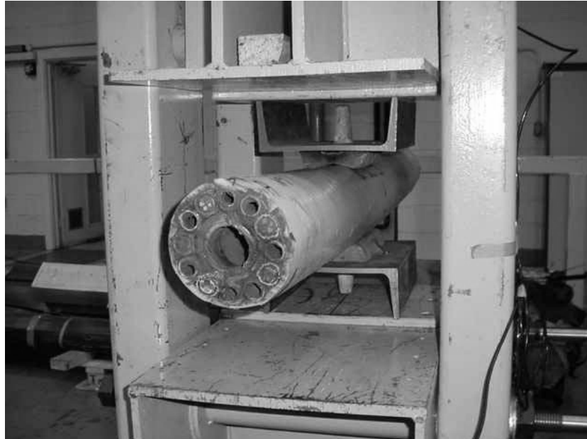
Figure 11. DUCO crushing test.
