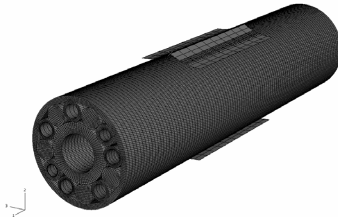
Figure 12. FE model of the crushing test.
