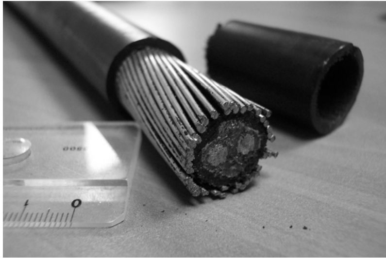
Figure 15. Armoured electrical cable used in the umbilical.
