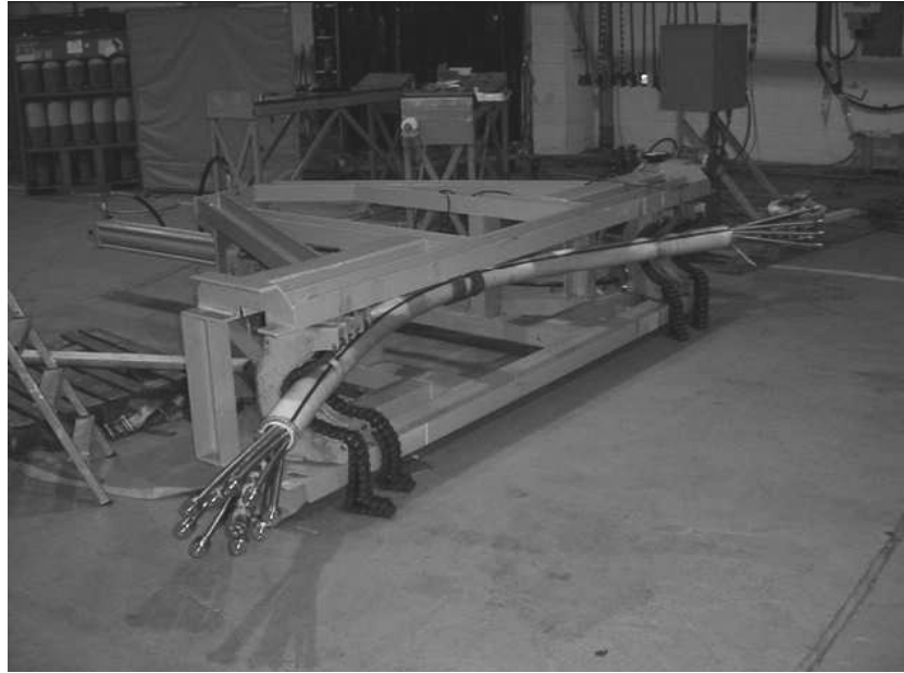
Figure 6. DUCO three point bending test rig.
