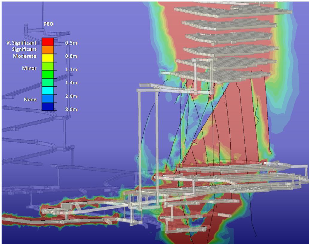
Figure 7. P80 (size of the 80<sup>th</sup> percentile fragment) on a section through an entire cave column.
