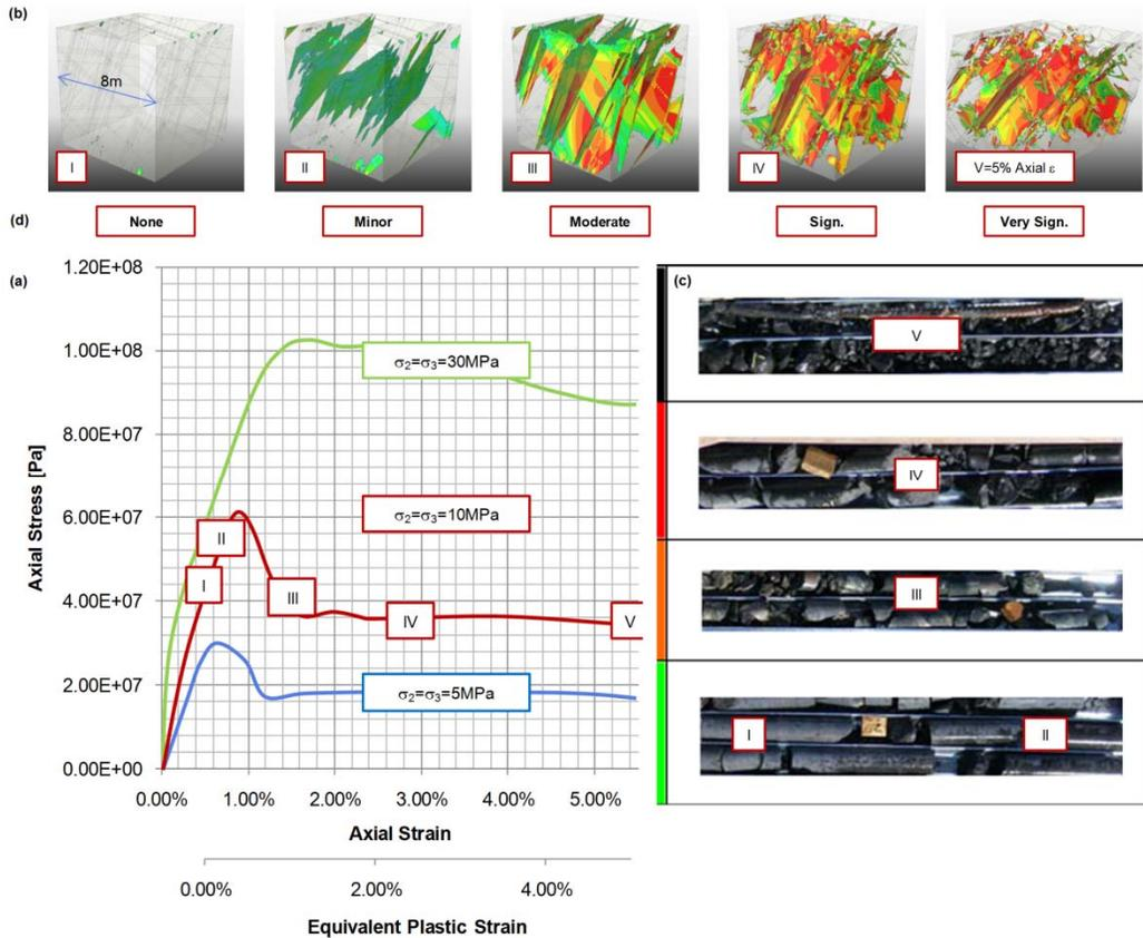
**Figure 4. Comparison of (a) Stress-strain response of a simulated rock mass specimen (8m diameter) at varying levels of confinement. (b) The yield state of discontinuities and the deformation of the specimen at milestones of yield (c) photographs of diamond drill core specimens, simulated by the global model to be at (d) respective states of strain on the Common Damage Scale.**
