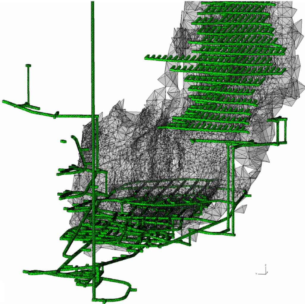
**Figure 1. Mesh of a mine scale model geometry with a geological domain outlined.**
