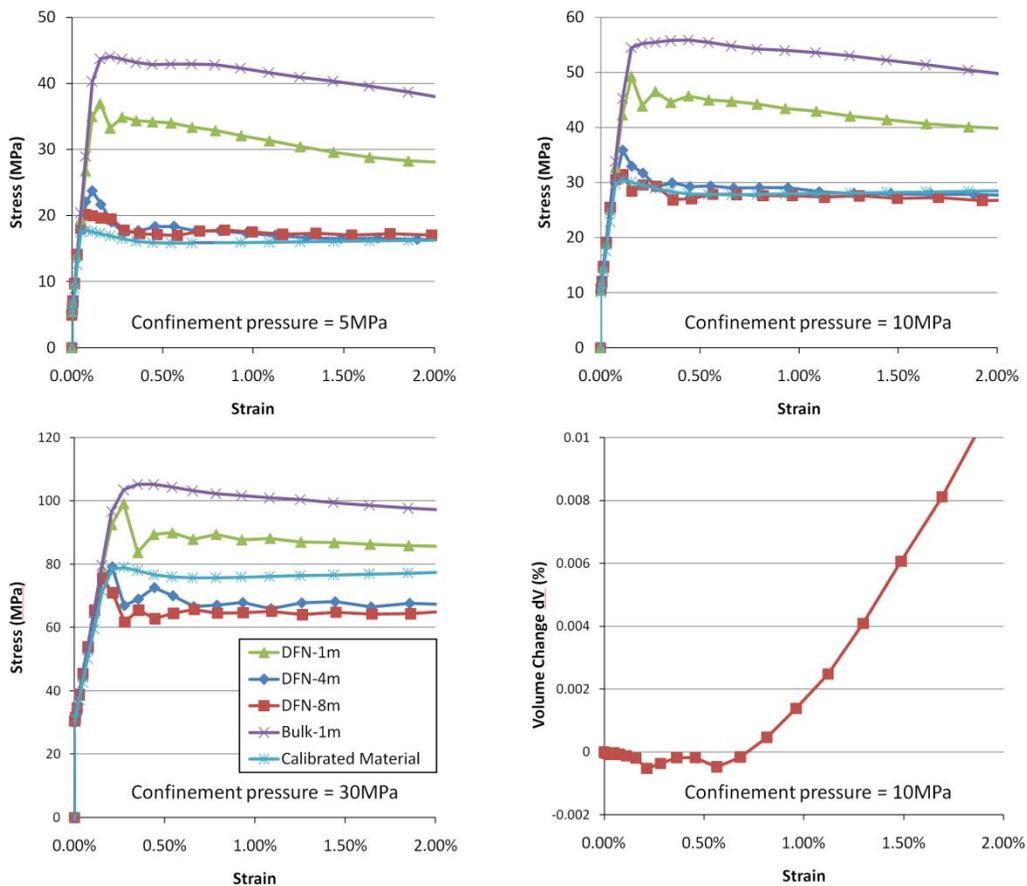
**Figure 3. Size and confinement effects in uniaxial DFN tests.**
