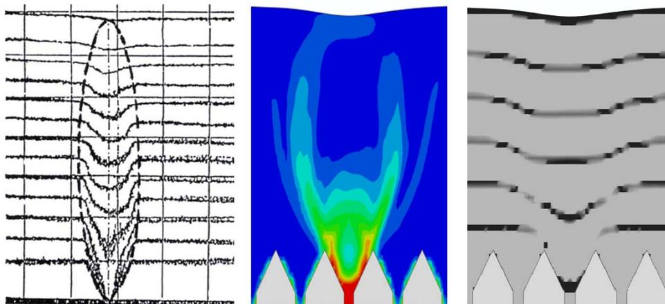
**Figure 8. Zone of loosening in sand model (Kvapil, 1965, left) and eulerian analysis (middle, right)**
