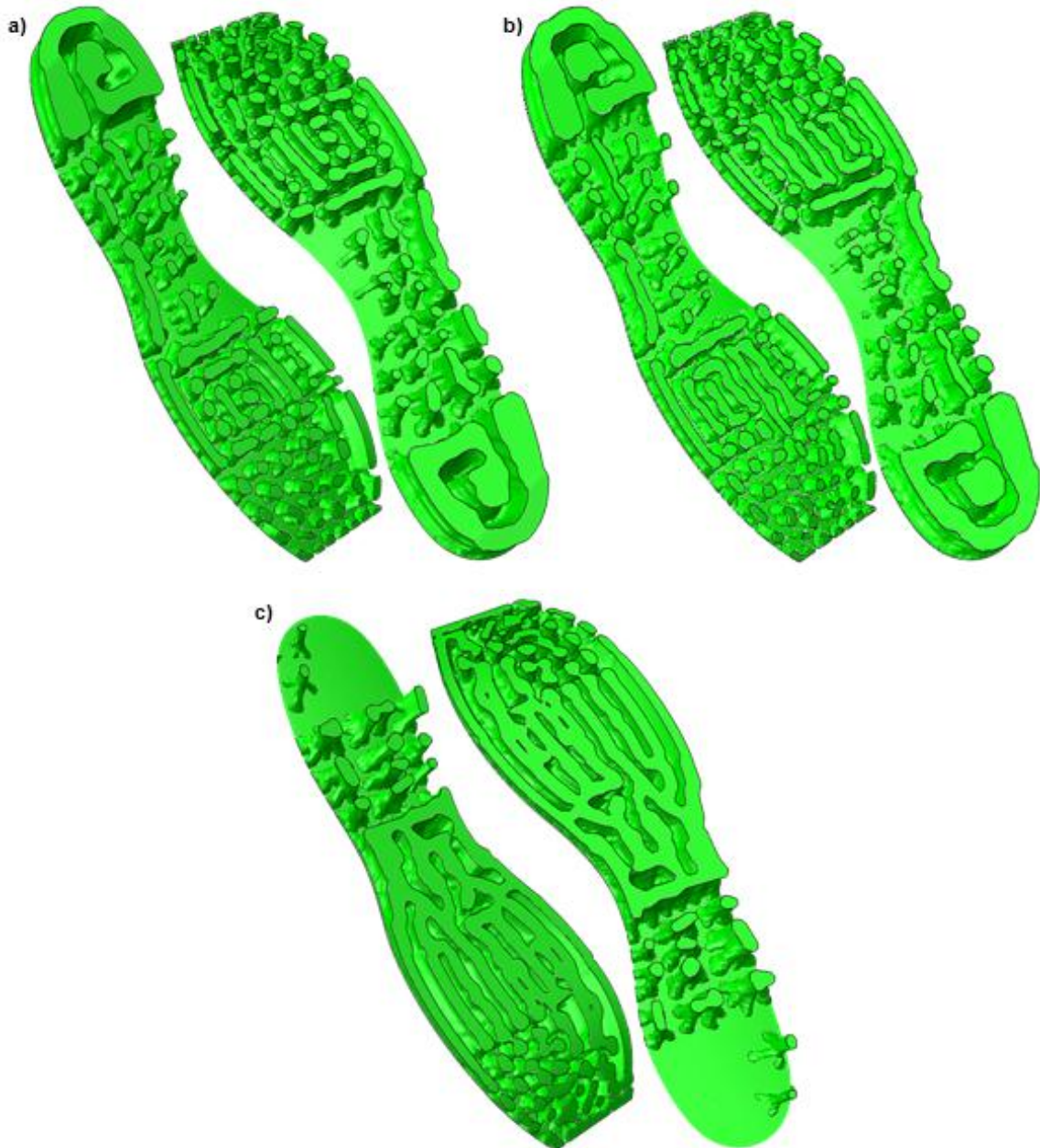
Figure 2. Optimised midsole geometries output for each subject. a) Subject A (rearfoot striker), b) Subject B (rearfoot striker), and c) Subject C (forefoot striker).
