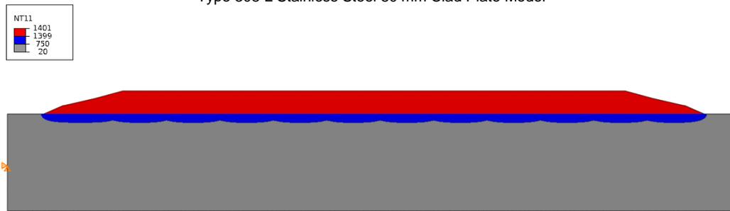
Type 308 L Stainless Steel 40 mm Clad Plate Model
