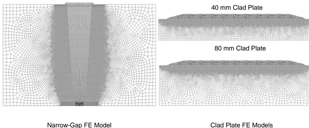
**Figure 2. Finite Element Model Meshes for Simulation.**
