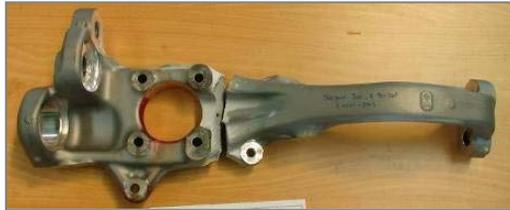
Figure 4. Failure mode of CA case fatigue test.
