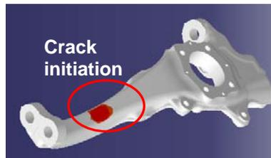
**Figure 11. Crack initiation area of MA2 and MA3 case.**
