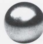
Hard grind polishes balls
