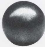
Soft grind removes flashing
