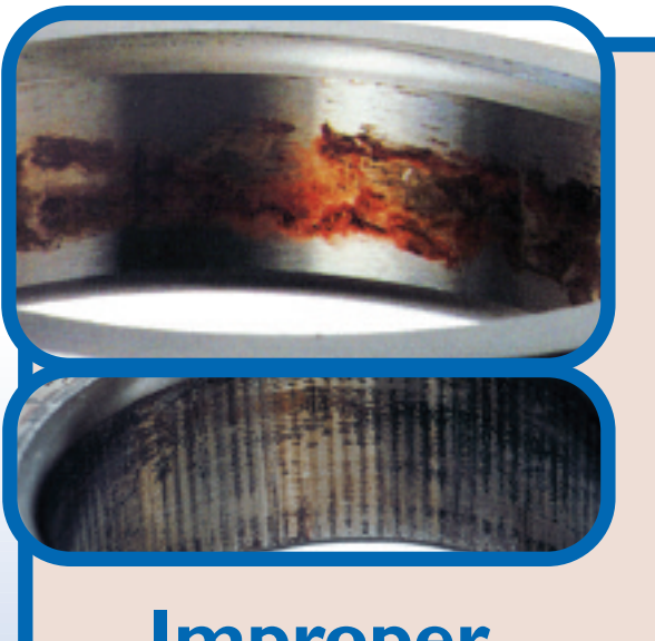
Improper Inner Ring Fit
