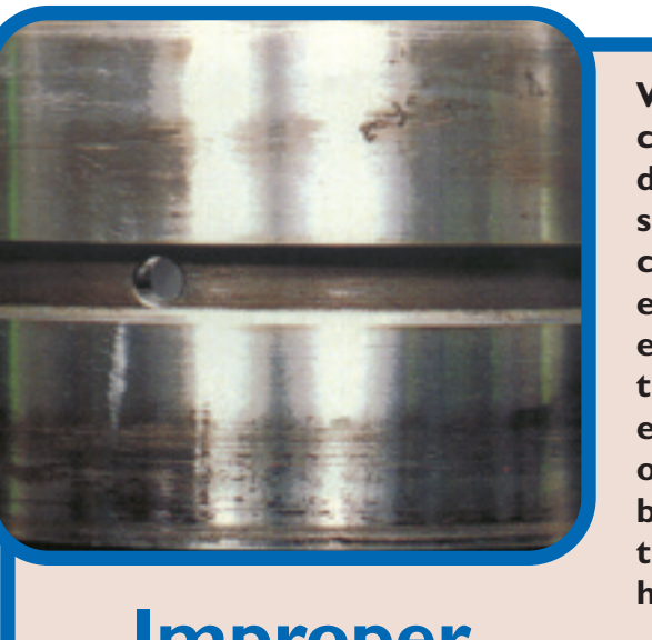
Improper Outer Ring Fit
