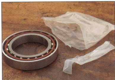
Don't open bearing pouch until ready to assemble components.
