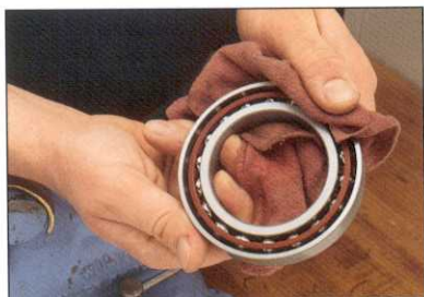
Don't wipe parts dry with a rag, or lint could be introduced into the bearing.
