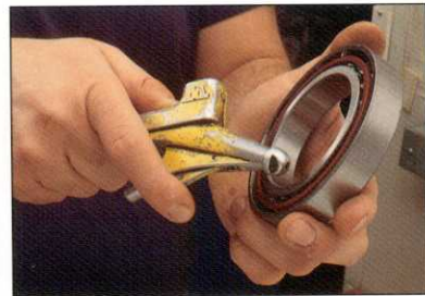
Don't spin bearings with compressed air. Internal damage could result.
