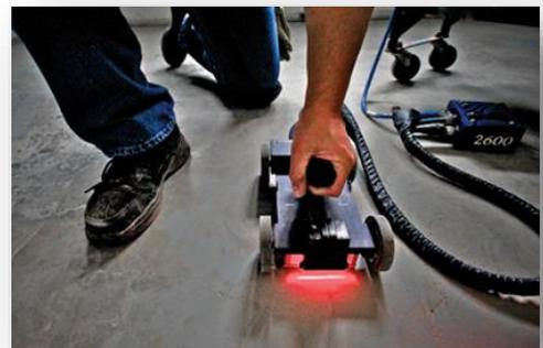
For [concrete structure scanning](#) our portable systems operate on frequencies of 1GHz, 1.6GHz, and 2.6GHz. We also have a very compact system for getting into tight corners with a frequency of 2GHz.
