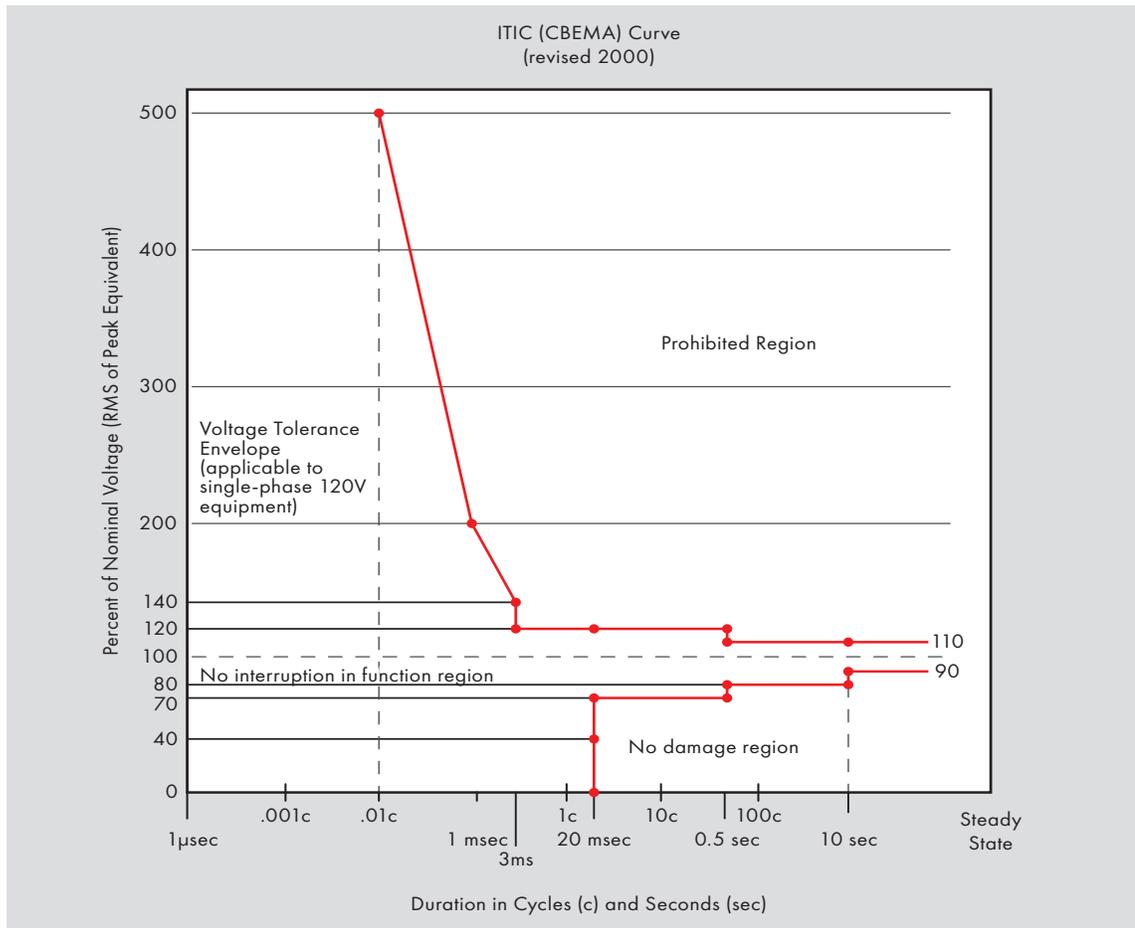
Figure 2. The ITIC curve is a modified version of the CBEMA curve.
