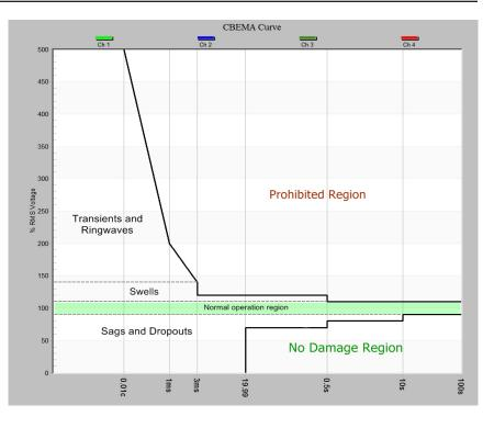
**Damage Region.** Events in this region include sags and dropouts of longer duration than those specified in the preceding event descriptions. This region also pertains to steady state voltages less than 90% of RMS nominal voltage. Normal functioning of connected equipment is not expected but no damage should result.
