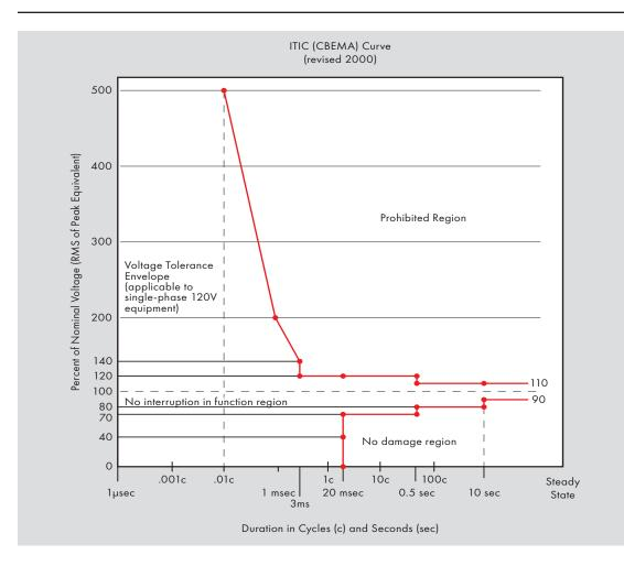
Figure 2. The ITIC curve is a modified version of the CBEMA curve.
