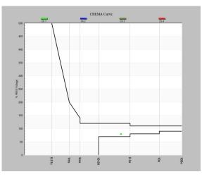
Figure 5. The event shown in Figure 4 does not exceed ITIC limits.
