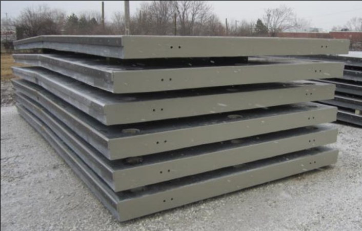
Deck has the crown molded into panel shape
