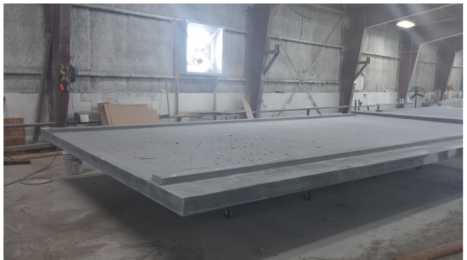
Molded deck panel with integral spacers prior to finishing work.
