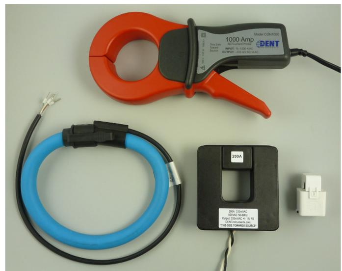
Figure 3: Current transformers available with the ELITEpro.
