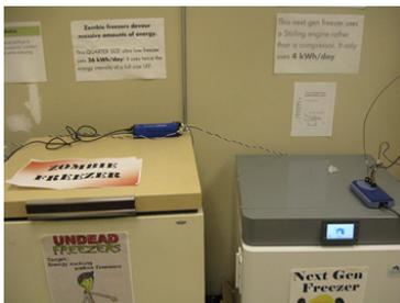
Figure 1: Two of the freezers in UC Davis' biology labs, with DENT Instruments' ELITEpro power meters installed. The wall signs show that newer, more energy efficient freezers consume significantly less power than older, less efficient ones (4kWh versus 26 kWh per day).
