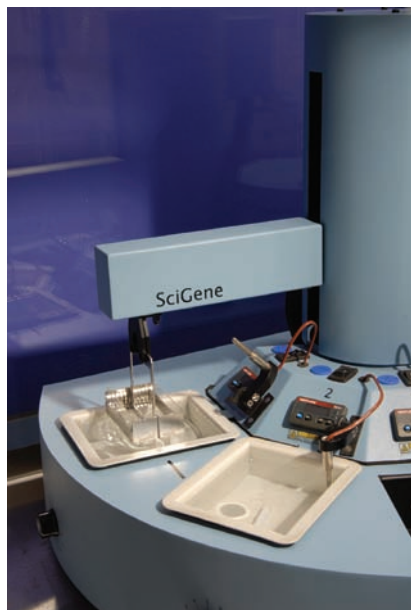
Figure 3 Automated washing and drying eliminates degradation of fluorescent dyes and potential variability in data results. System from SciGene (Sunnyvale, CA).
