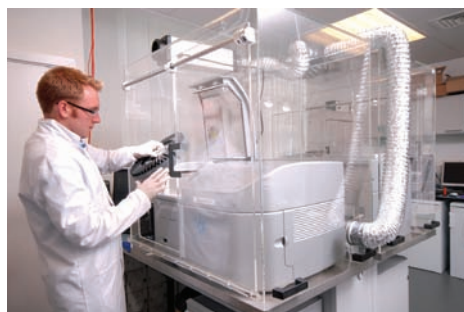
Figure 4 OGT utilizes an ozone-free cabinet, which is important for detecting gene expression measurements since environmental ozone can degrade cyanine 5 (Cy5) in microarrays.
