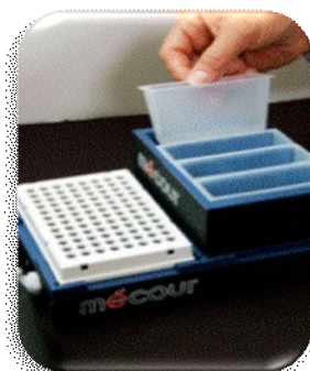
Easy loading of reagent reservoir to Thermal Insert
