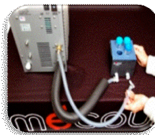
Align thermal block for connection.
