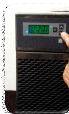
Set desired circulator temperature setting.
