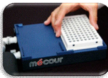
Load plate/insert on thermal block.
