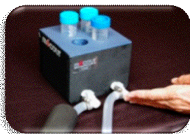
Insert fluid Quick Disconnect to thermal block.
