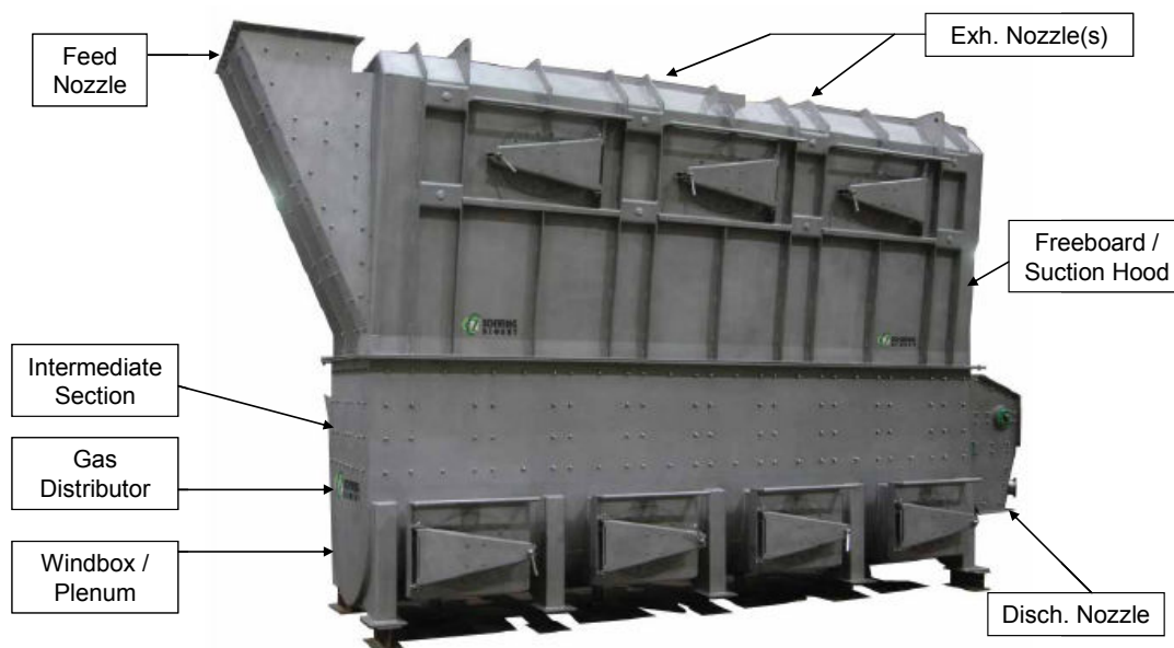
Figure 4: Fluidized Bed Unit Major Components
