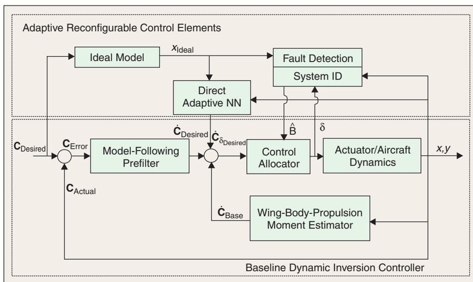
Figure 9. Dynamic-inversion-based adaptive/reconfigurable control system.
