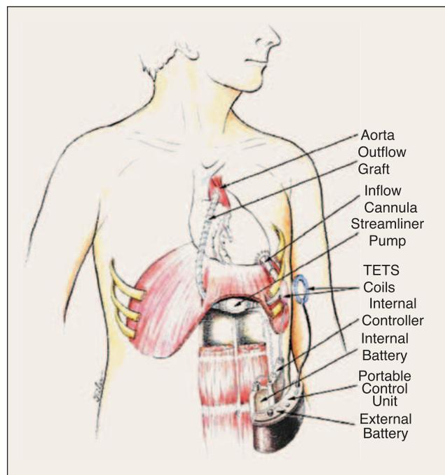
**Figure 1.** Configuration of the Streamliner artificial heart system as planned for implantation in humans.
