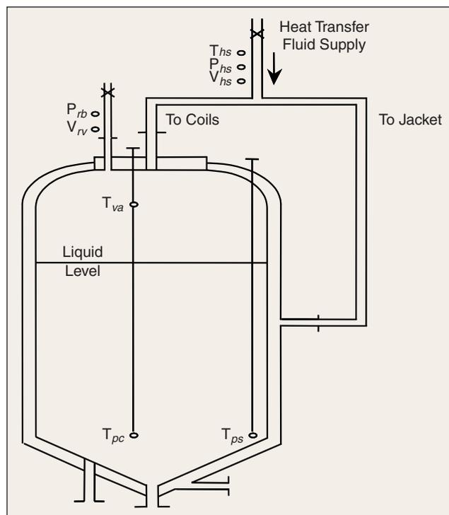
Figure 7. Example of a batch chemical process reactor.
