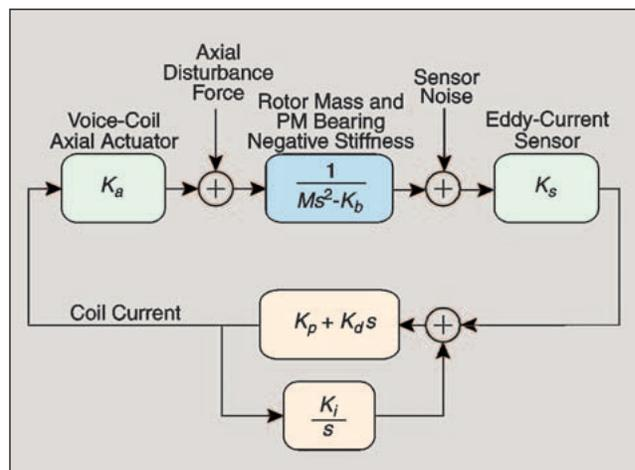
**Figure 4.** Axial controller block diagram for Streamliner artificial heart. The transfer function from disturbance to control current has a zero at dc. This is known as a virtual zero power (VZP) controller in the magnetic bearing community.
