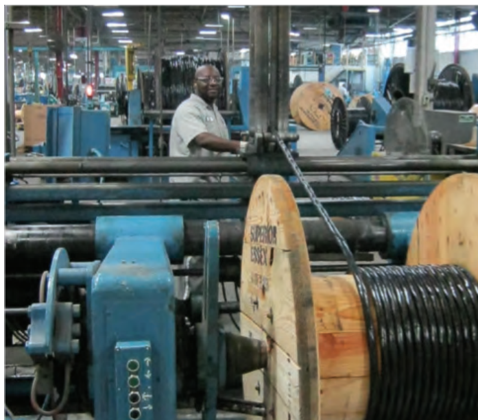
Picture of cable being re-spooled from large reel to smaller reel
