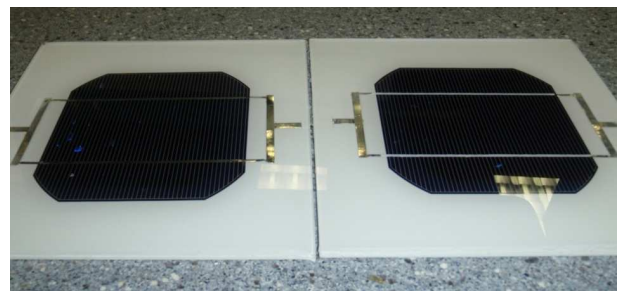
Fig. 4: (Left) Photograph of a mini-module with typical, specular reflective metallic bus wire. (Right) Diffuse reflective bus bar.
