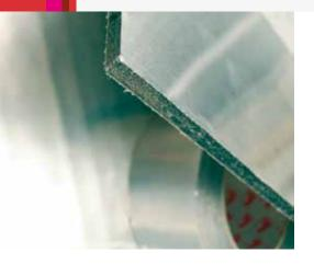
DuPont<sup>™</sup> Energain comes in aluminiumlaminated sheets that can be cut to any size. Once cut, aluminium tape is used to seal the edges of the sheets and to cover any holes or abrasions that may occur during installation.
