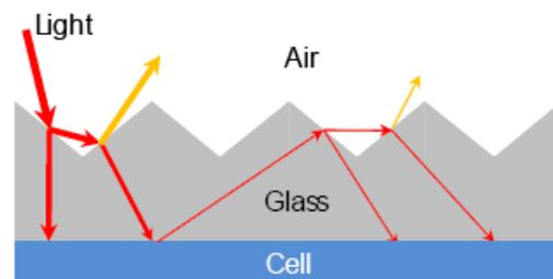
**Figure 2:** Interaction of light at the air-glass interface for structured glass.
