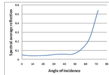
**Figure 1:** Effect of angle of incidence on spectral reflection.
