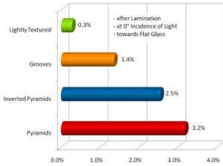
**Figure 6:** Percentage increase in  $I_{sc}$  for normally incident light.
