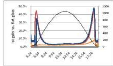
**Figure 11:** Gain in  $I_{sc}$  of structured glass modules relative to reference module: Grooves (red), pyramids (blue), and lightly textured (orange). Irradiance (black,  $W/m^2$ ) is also shown. Sharp peaks near 7:00 AM are due to discontinuous measurements recorded by the DAQ system. Data is from August 13, 2010.
