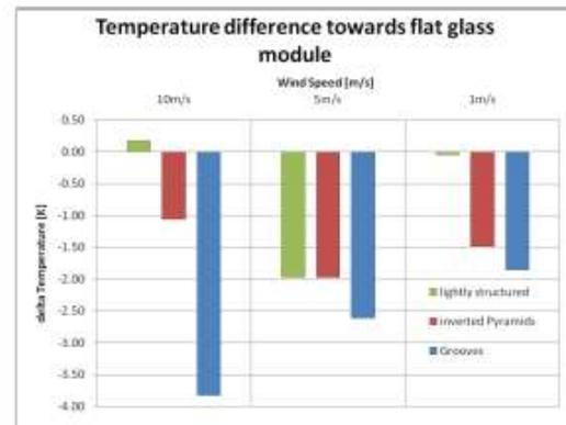
**Figure 9:** Effect of wind speed on module temperature
