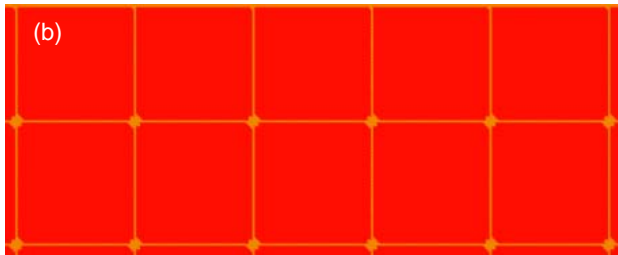
Figure 9: Temperature mapping of a PV module after 1 hour outdoor exposure to sun obtained from (a) thermal imaging and (b) EMW model. The same colors are used in each profile. The street region appears more distinct in the EMW model due to the relatively large size of the elements.
