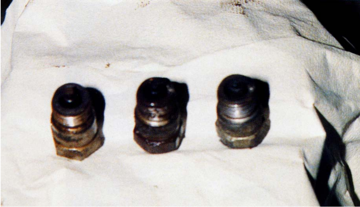
Photograph 5 – Spark Plug Deposits - Before
