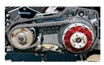
We've already talked about the importance of clean oil and a clean air filter in your bike's health. But another essential part that works with these components is the chain, belt or shaft that enables your transmission to drive your bike's wheel – the drivetrain. Which one of these you have depends on the model of bike you have.
