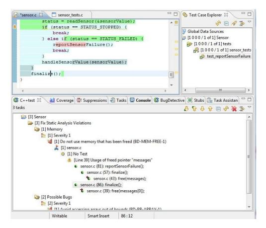
A potential path—one that was not covered—is discovered in which a double free in the finalize() function is possible. The reportSensorValue() function calls finalize(), then the finalize() calls free(). Also, finalize() is called again in the mainLoop(). We could fix this by making finalize() more intelligent, as shown below:
