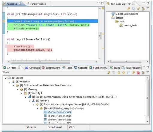
This indicates reading an array out of range at line 48. Obviously, the msgIndex variable must have had a value that was outside the bounds of the array. If we go up the stack trace, we see that we came here with this print message with a value that was out of range (because we put an improper condition for it before calling function printMessage()). We can fix this by taking away unnecessary conditions (value <= 20).
