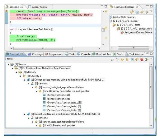
Our test case uncovered more memory-related errors. We have a clear problem with memory initialization (null pointers) when our failure handler is being called. After further analysis, it's clear that we mixed an order of calls in reportSensorValue(). The finalize() function is being called before printMessage(), but finalize() actually frees memory used by printMessage().
