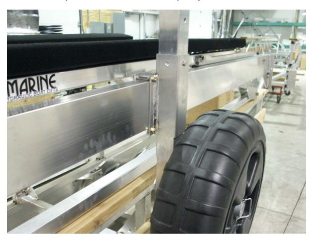
3. Photo below shows (2) pair of Wheel Kits attached to the Front and Rear Beams.
