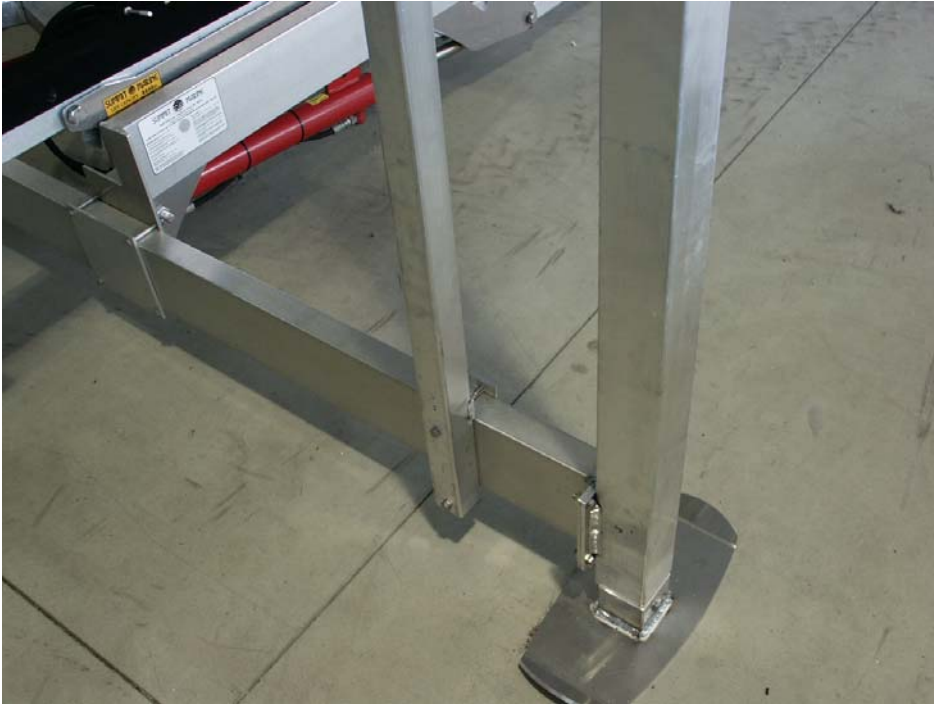
Wrong location – Upright Post is facing outside the lift beam.
