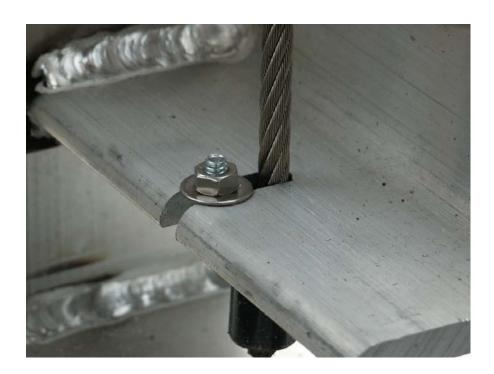
19: The winch corner ('Bed A') will have an unfinished cable end. Feed this end up into the winch hub as shown. Note the direction of the cable. Thread through the hole until it is flush with the exit hole. Fasten with  $5/16 \times .5$ " set screw from Bag 4 into hole shown, tighten.
