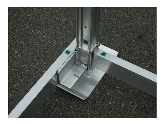
4: At the bottom of the Corner Post, slide (1) square nut, (1) washer, and (1)  $3/8 \times .75$ " screw into the small channel, hand tighten about 7" from the end. Repeat for the other channel, and repeat for the other (3) Posts. Totaling (8) screws. (2) in each post. These screws will be retightened over the top of the Base Beam slot in the next step.
