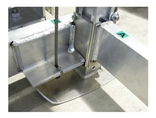
17: Attach the (5) upper cables as shown. The Horizontal Brace side will have (2)  $\frac{1}{4}$ " x 2" square plates to run the cables through. You may want to lift the bed slightly to facilitate this step. Screw the  $\frac{1}{2}$ -13 nuts onto the screw ends. Level the bed, and snug the screws without over tightening. Too tight and the Bed will tilt down toward the winch, too loose and the Bed will tilt up toward the winch. Jam the second  $\frac{1}{2}$ -13 hex nut on the screw.
